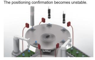
After PE switch mounted on the table Positioning confirmation accuracy is improved.
