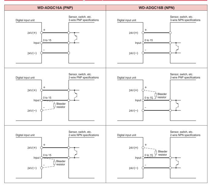
If using a sensor with a lower limit value of load current that exceeds the specification value of the input current, connect a bleeder resistor to increase the sensor load current. 12 k $\Omega$  (1/10W and over) load current increases by approx. 2 mA by connecting the bleeder resistance.
